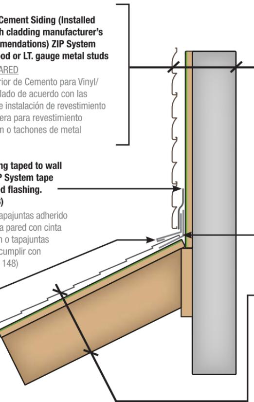
**ZIP System tape sealed between ZIP System wall Sheathing and ZIP System roof sheathing**
