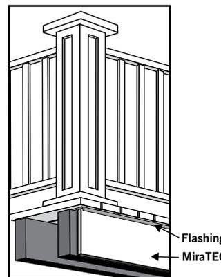
When vertical trim meets flashing at the top of trim or siding, provide a 1/4" clearance from the bottom of the trim to the top of the flashing.
