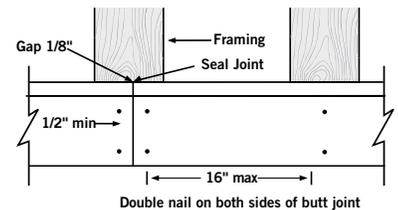
Double nail on both sides of butt joint
