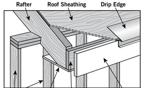
\* **Note:** Nail at least 1/2" from the edge. Do not nail into the edges of MiraTEC trim. For 4/4 and 5/4 fascia and soffit applications, MiraTEC trim can be fastened directly to the rafter ends, double nailed a maximum of 24" on center. For 5/8" fascia and soffit applications, MiraTEC trim must have a sub-fascia and be nailed 16" on center to the rafter ends or sub-fascia. For all other horizontal and vertical applications, double nail 16" on center, falling on the studs.
