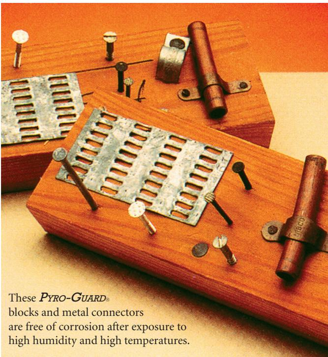
These *PYRO-GUARD*® blocks and metal connectors are free of corrosion after exposure to high humidity and high temperatures.
