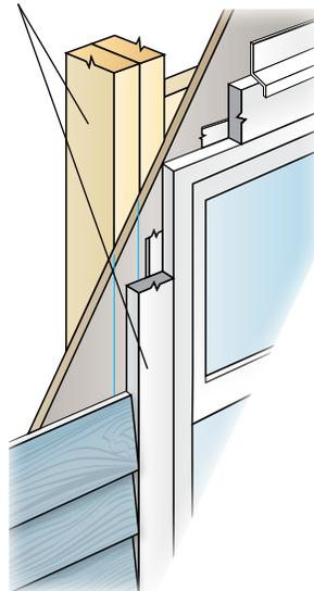
Notch plank around window trim and flashing.
