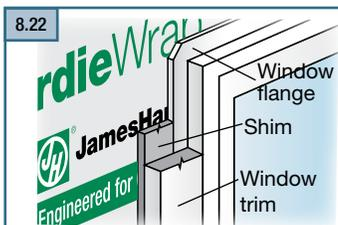
**TIP:** For trimming around windows and doors with attachment flanges, install a shim strip to build out the wall even with the flange. This strip lets the trim sit flat and parallel with the wall.
