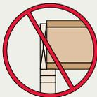
**DO NOT** use sawn lumber for rim board or blocking as it may shrink after installation. Use only engineered lumber
