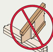
TJI® joist flange must bear fully on the plate. See detail BC on page 15.
