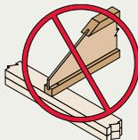
**DO NOT** bevel cut joist beyond inside face of wall.
