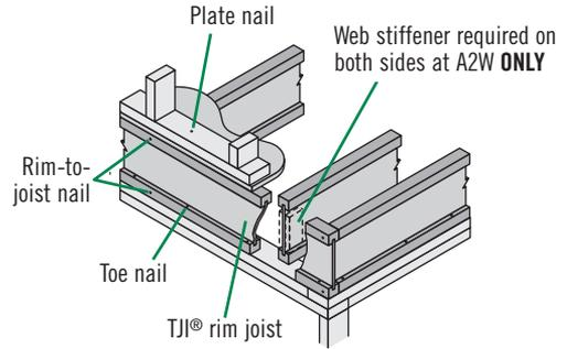
**A1** **A1W** Attach blocking per A3.1 in rim board installation table above
