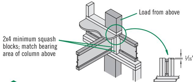
**CS** Use 2x4 minimum squash blocks to transfer load around TJ® joist
