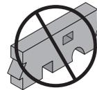
**DO NOT cut, notch, or drill holes in headers or beams except as indicated in the illustrations and tables.**
