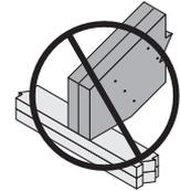
**DO NOT overhang seat cuts on beams beyond inside face of support member**
