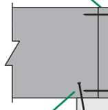
Drive nails at an angle to minimize splitting of plate
