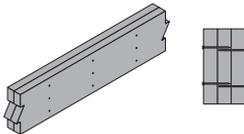
**L6** Multiple pieces can be nailed or bolted together, up to a maximum width of 7"
