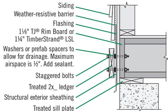
**LA** Corrosion-resistant fasteners required for wet-service applications
