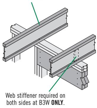
**B2 B2W** Blocking panels may be required with braced/shear walls above or below—see detail B1
