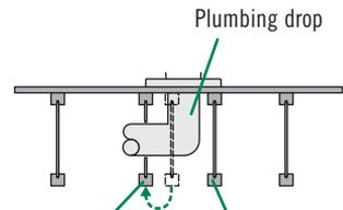
Joist may be shifted up to 3" if floor panel edge is supported and span rating is not exceeded. **Do not cut joist flanges.**
