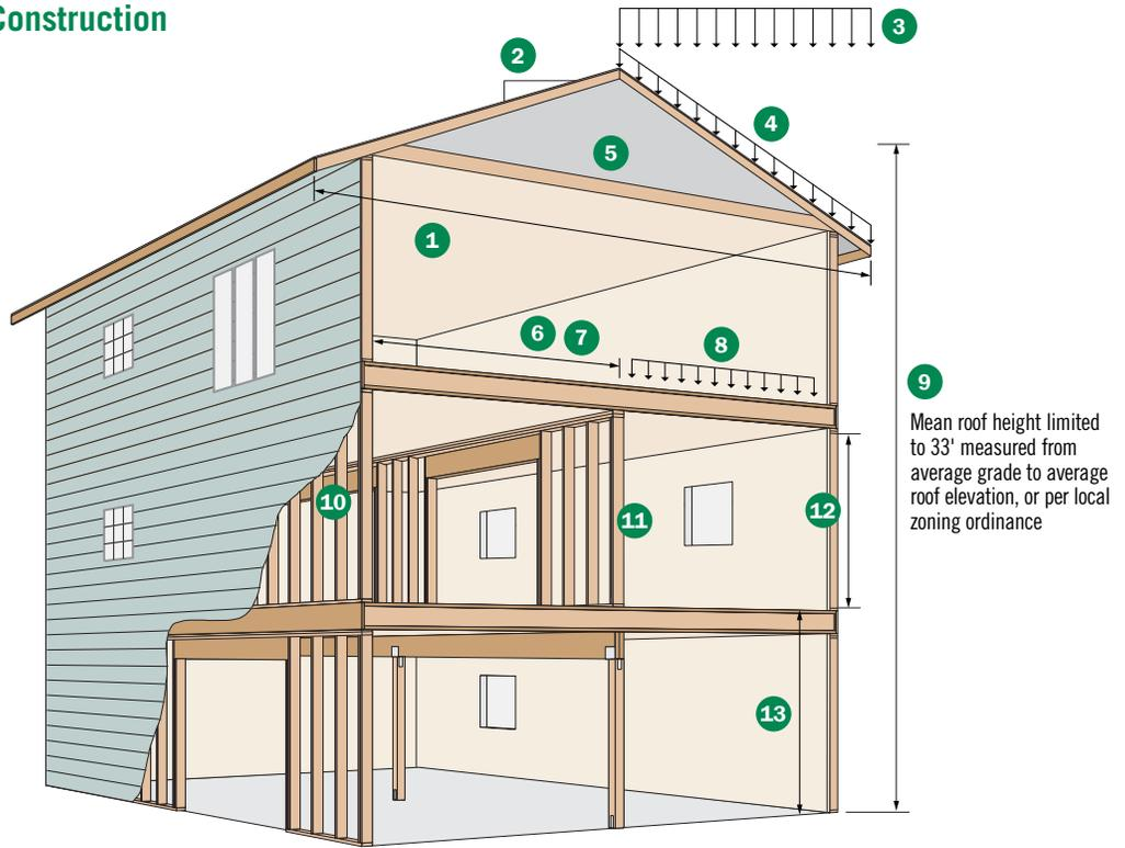
9 Mean roof height limited to 33' measured from average grade to average roof elevation, or per local zoning ordinance
