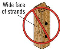
DO NOT install bolts or screws into the narrow face of strands
