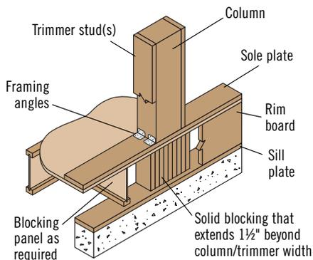
**P5** Solid blocking that extends 1 1/2" beyond column/trimmer width is required if column and trimmer studs do not extend to sill plate
