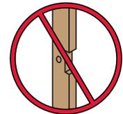
**DO NOT cut a notch and a hole in the same cross section**
