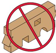
**DO NOT cut, notch, or drill holes in headers or beams except as indicated in the illustrations and tables above**
